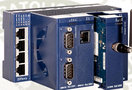
Figura 4.46. Router VPN Industrial Flexy 201 – eWON
