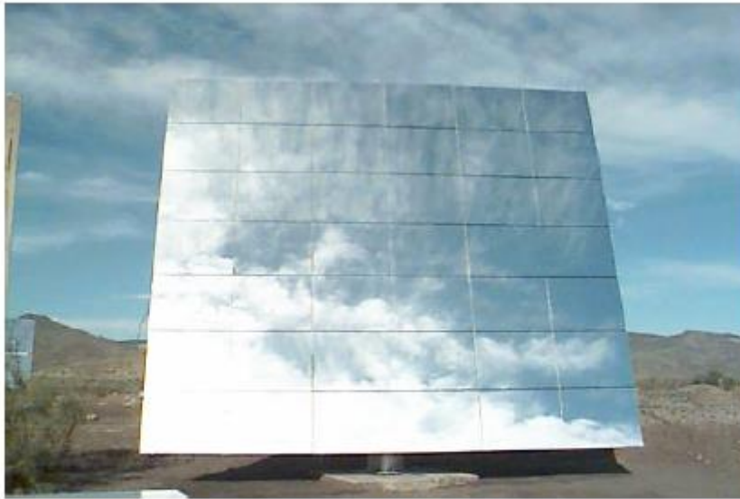
Figure 3. Front View of the Colon 70 Heliostat on test at the PSA in Almeria, Spain
