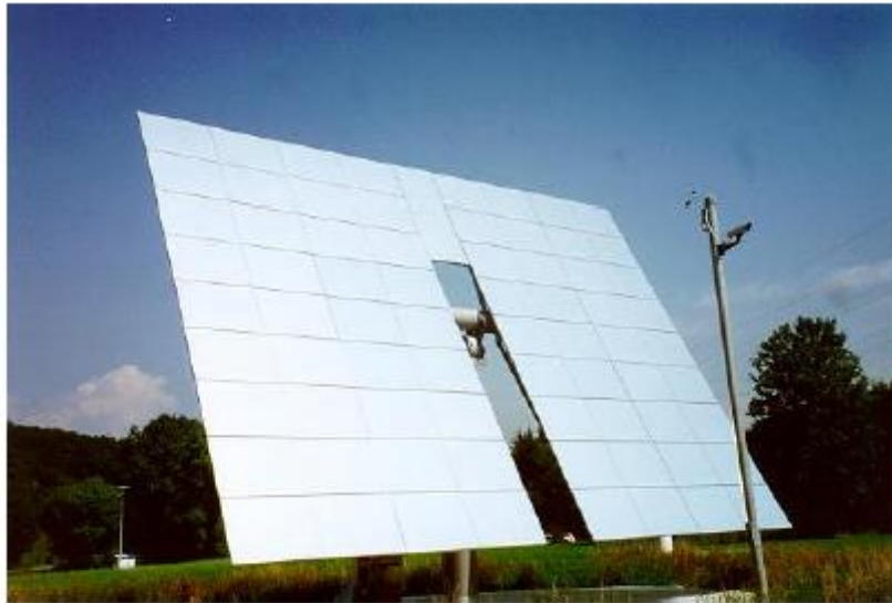
Figure 6. Front view of the PSI 120 heliostat.
