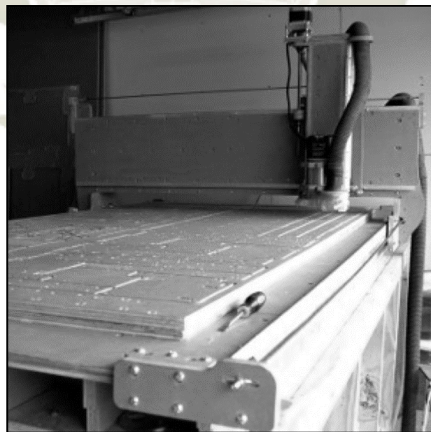
Figura N° 25. Router CNC 4'x8' Heavy Duty - CNC Machine Kit (greenBull 4X). Fuente: https://buildyourcnc.com/Item/cnc-machine-greenBull-v4-4X-milling
