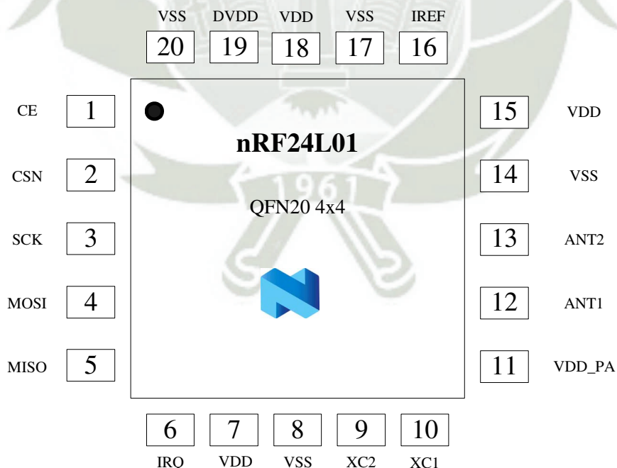
Figure 2 nRF24L01 pin assignment (top view) for a QFN20 4x4 package.
