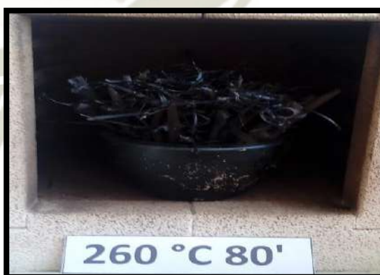
Figura 14. Biomasa torrefactada 260°C 80' (T2t1)
