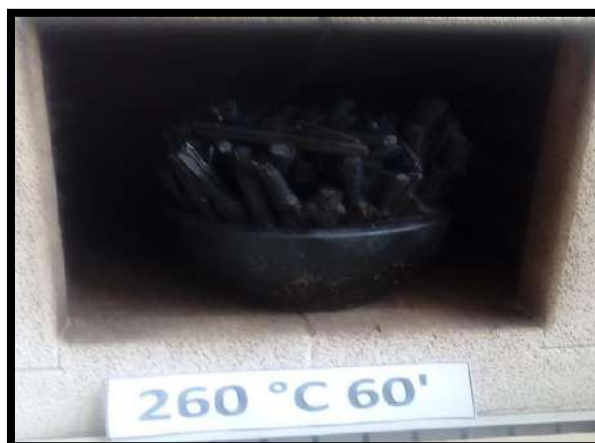
Figura 15. Biomasa torrefactada 260°C 60' (T2t2)
