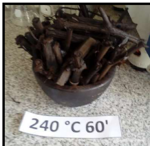
Figura 18. Biomasa torrefactada 240°C 60' (T3t2)
