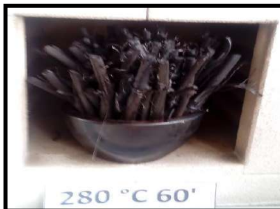
Figura 12. Biomasa torrefactada 280°C 60' (T1t2)
