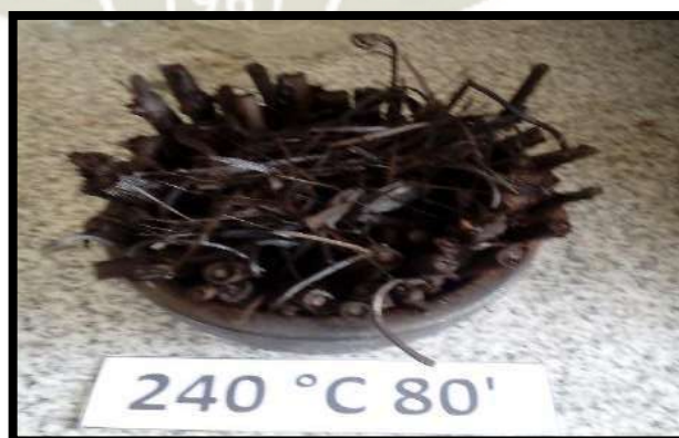
Figura 17. Biomasa torrefactada 240°C 80' (T3 t1)
