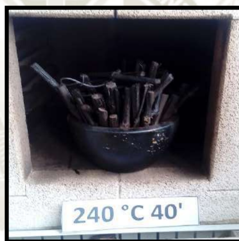
Figura 19. Biomasa torrefactada 240°C 40' (T3t3)
