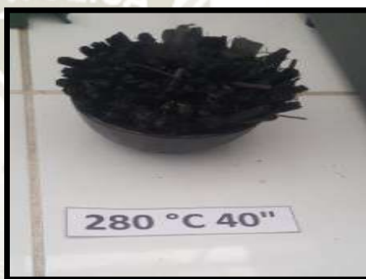
Figura 13. Biomasa torrefactada 280°C 40' (T1t3)
