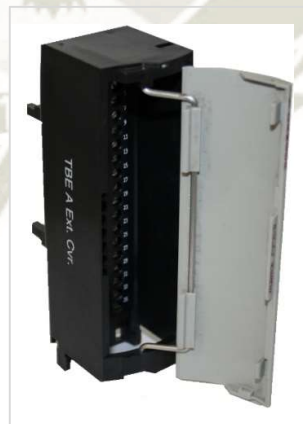
Fig. 40 Base terminal Contrologix. 1756-TBCH.
