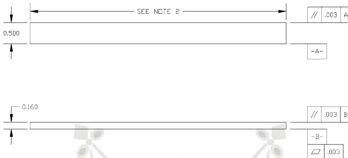
FIG. 5 Standard Flexural Test Specimen Drawing (Inch-Pound)
