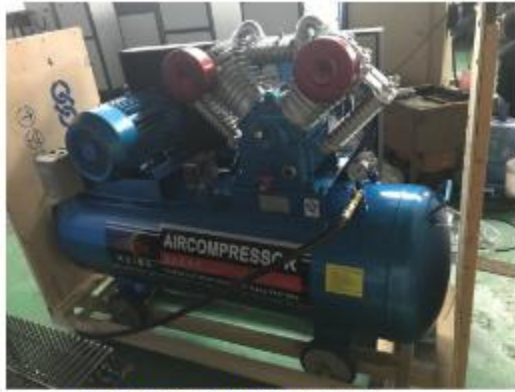
High pressure Air compressor
