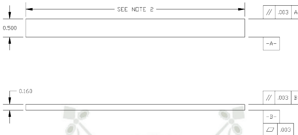
FIG. 5 Standard Flexural Test Specimen Drawing (Inch-Pound)
