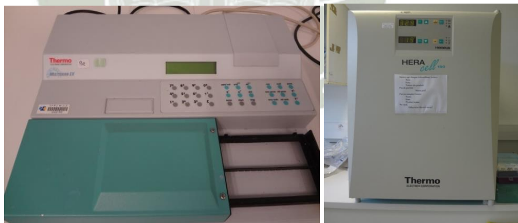
Fig. 10 Thermo Scientific Multiskan EX (lector de placas), incubadora The Heraeus® HERAccl® by Thermo Electron.
