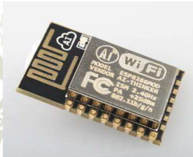
Figure 3 [Module Pin Counts, 22 pin, 16 mm *24 mm *3 mm]
