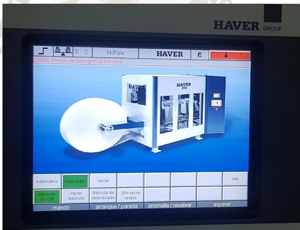
Figura 84. Panel de control Ensacadora HAYER (Planta Prillex 2017)
