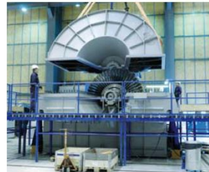
SST-900 steam turbine in the workshop in Finspong, Sweden.
