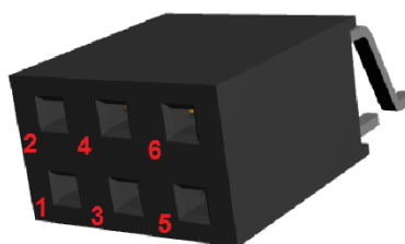
Figure 14: Pinning SPI connector CON3 and CON4
