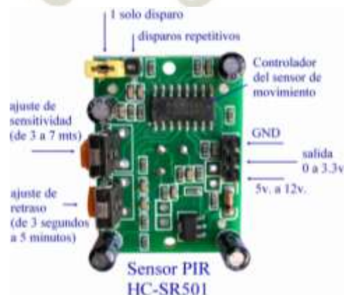
Figura 2. Sensor PIR HC-SR501
